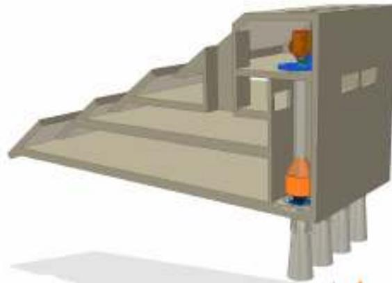
**Figure 2.** SSG pilot plant at Kvitsøy Island, 3-level reservoirs. Below, drawing of the device with view of the low-head turbines.
